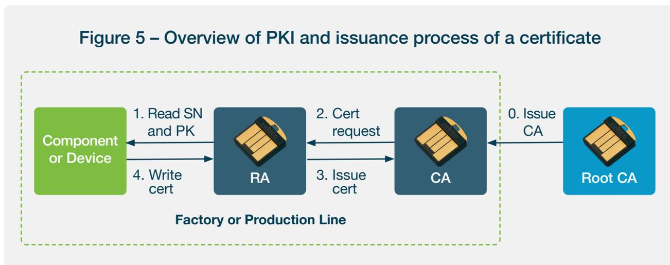
Under the illustrated design, the Root CA uses a YubiHSM 2 to house its key-pair (i.e. both its Private and Public Keys) in addition to its certificate. Due to the diminutive size of the YubiHSM 2, the Root CA server can practically be located anywhere, although traditionally, the Root CA is hosted in an offsite data centre for security reasons, but also due to the tremendous physical size of server farms and a typical HSM.
