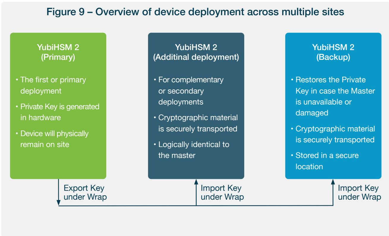
Relating the replication concept back to the JTAG use case covered previously in this paper, one YubiHSM 2 device could be deployed directly to a production line for writing encrypted serial numbers to the ECUs, while another device could be delivered to a trusted customer for unlocking the corresponding JTAGs for testing. Another device still, could be stored in a safe as backup, in the event the primary device is lost, stolen or damaged.
