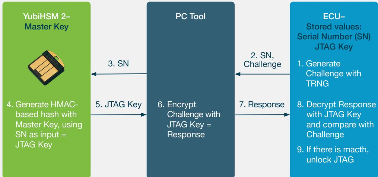
Now, before a symmetric mechanism can even be employed, manufacturers need to generate both the Serial Numbers and JTAG Keys, record the issued Serial Numbers, and finally, deploy the JTAG Keys to the relevant ECUs. *Figure 4* (below) summarises the process of how manufacturers might generally be able to accomplish this, using a HMAC-based cryptographic algorithm—or a YubiHSM 2, as the case may be.
