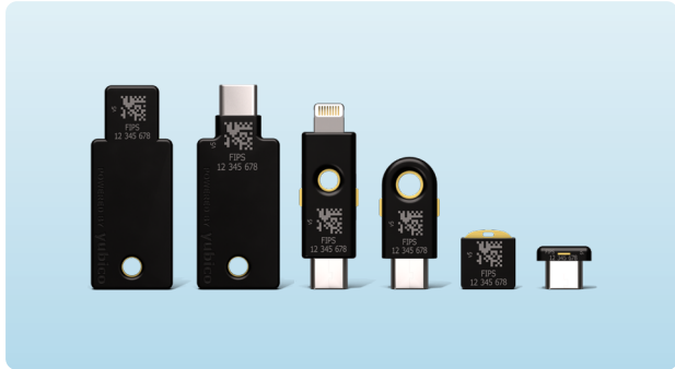
The YubiKey FIPS series—from left to right: YubiKey 5 NFC FIPS, YubiKey 5C NFC FIPS, YubiKey 5Ci FIPS, YubiKey 5C FIPS, YubiKey 5 Nano FIPS and YubiKey 5C Nano FIPS
