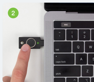
2 LED blinks green and checks for matching user fingerprint.
