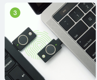
3 LED stops blinking when user successfully authenticated.
